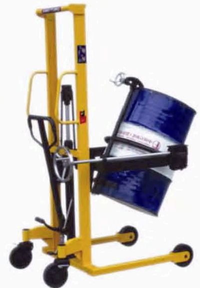
WONT Hyd. Drum Lifter Cum Tilter Model : W-HDLCT Capacity : 400 Kg. Lift Height : 1.5 / 2.0 / 2.5 / 3.0 mtr.
